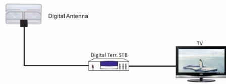
1. Connect the aerial lead either directly to the back of your Digital TV [Fig.1] or Terrestrial STB [Fig.2] as shown in the diagrams above.
