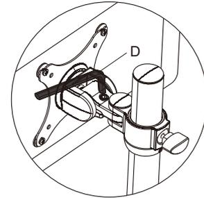
To adjust the screen angles use the 5x5 allen key supplied
