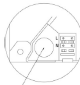
Hole for the insertion of the electric ducting.
