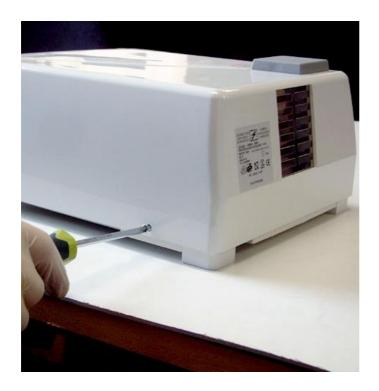
Remove the casing from the base.
