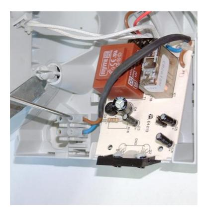
Remove the electronic circuit board from its position, freeing it from its clips and replace it. Fit it by following the previous steps in reverse order.
