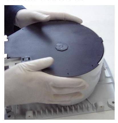
Remove the fan by loosening the nut that secures it to the drive shaft.
