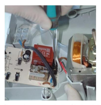
Disconnect the two power supply cables of the electronic circuit board that go to the terminal block that is connected to the grid.
