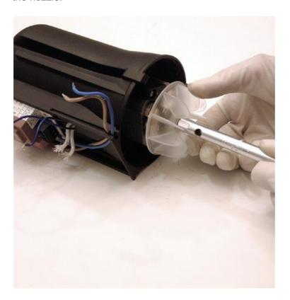
Unscrew the motor from the turrets inside the nozzle.
