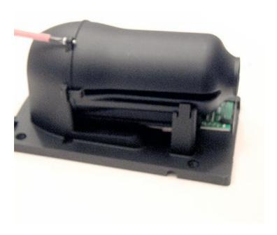
Open the nozzle by releasing the clips that secure it to the base.
