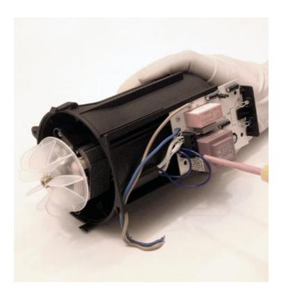
Disconnect the two heating element cables that go to the electronic circuit board (two white cables).
