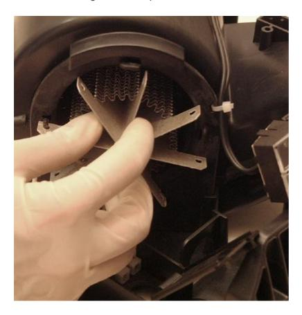
Carefully remove the heating element from its position.
