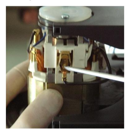
Remove the brush from its location and replace it. Carry out the same procedure for the second motor brush.
