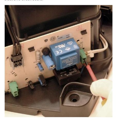
Carefully remove the electronic circuit board from the guide in the base by bending the clips located in the volute.
