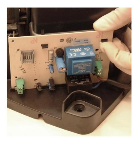
Remove the circuit board carefully so as not to damage its components. Fit it by following the previous steps in reverse order.
