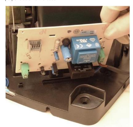
Position of the jumper at low sensitivity: detection distance between 15 and 20 cm.
