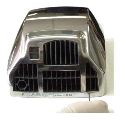
The casing is fixed to the base by means of inner bolts. Extract the lower part of the casing, as shown in the image, and lift it slightly to release the anchors.
