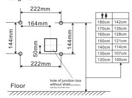
The power cord Supplying the hand dryer should be at least 1.5m<sup>2</sup> 2 Core & Earth
