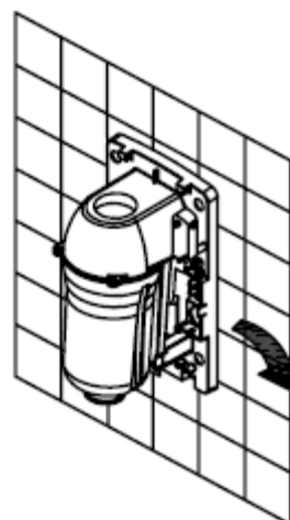
Terminal strip and 22-mm diameter entrance hole
