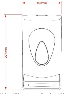
Height: 275mm Width: 150mm Depth: 130mm Capacity: 230mm Stack
