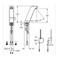
PROTRONIC-S mains-supplied washbasin mixer with touch-free operation, DN 15, noise group I, with aerator and integrated flow control, for connection to hot and cold water supply, polished chromium-plated brass. With temperature selection lever, conversion set for concealed mixing device and with power supply for installation in the wall, 230 V AC.
