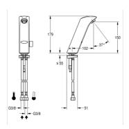
PROTRONIC-S battery-supplied washbasin mixer with touch-free operation, DN 15 with aerator and integrated flow control, for connection to hot and cold water supply, polished chromium-plated brass. With temperature selection lever and conversion set for concealed mixing device, 6 V battery.
