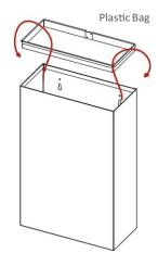
Height: 671mm Width: 344mm Depth: 167mm Weight: 6Kg Capacity: 30 Litre
