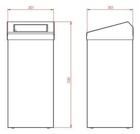
Height: 700mm Width: 301mm Depth: 301mm Weight: 7.5Kg Capacity: 50 Litre
