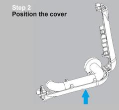
Open the cover fully and position the cover below the handle, making sure that the shaft is centrally aligned.
