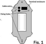
Unscrew the terminal enclosure, feed the mains cable into the enclosure, and connect the luminaire to the mains supply ensuring the correct polarity is observed (see Fig. 2):
