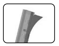
1. Peel off the 3M tape from the back of the LED strip
