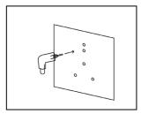
Drill the holes and insert the plastic hole plugs
