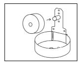
Install jumbo toilet roll. Install the inner spindle accessory if provided.
