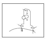
Secure the dispenser to the wall with the screws. It is recommended to use the top and the bottom holes. For added security use additional screw holes
