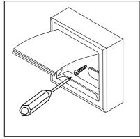
Fix the product to the wall using the provided screws or other suitable screws
