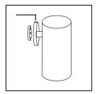
Using the allen key provided, remove the inner mounting plate from the fixing plate
