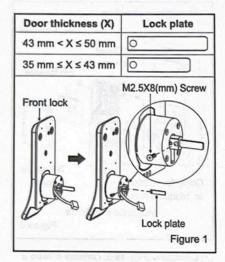
(1) As figure 1, Measure your door thick. If 43 < door thickness ≤ 50 mm, no need to change Lock plate.
