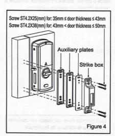
(4) As figure 4, Install strike box with 4 screws. (You can add/decrease auxiliary plates to adjust the strike box so that to align with the deadbolt.)
