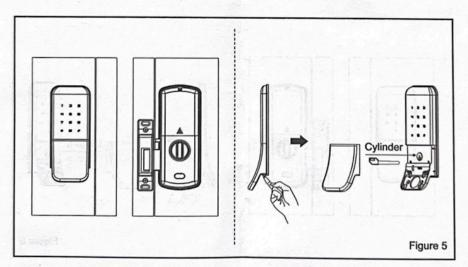
(5) As figure 5, Turn the knob to check if deadbolt work smoothly. Press the button (at the bottom) of the Front lock and take out the cylinder cover, use manual key to open and close the lock and check if deadbolt work smoothly.
