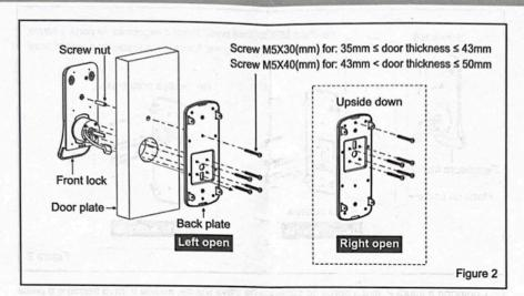
(2) As figure 2, Fix screw nut on Front lock, install Front lock and Back plate on door with 5 screws. Note: Figure 2 is Left open instruction, if you want to install as Right open, please turn the back plate upside down.
