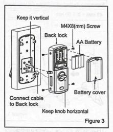
(3) As figure 3, Connect cable to Back lock, keep the lock plate vertical, and keep the knob horizontal. Use 4 screw to fix the Back lock on Back plate. (If door is Right open, please turn the back lock upside down)
