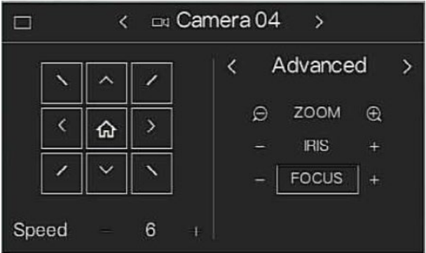
Figure 138 PTZ Control Panel
