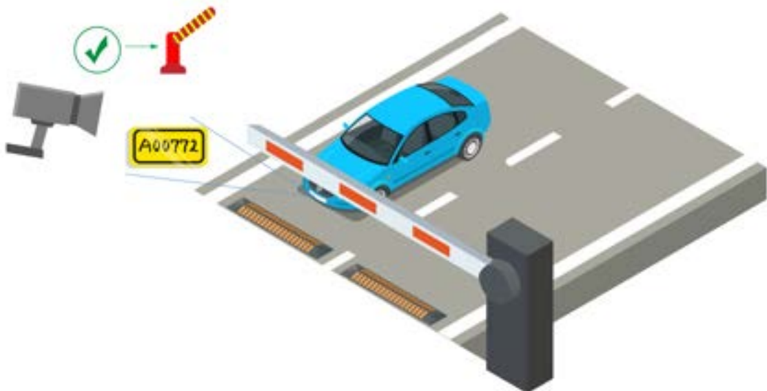
Figure 18-8 Example: Barrier Opened Automatically for Vehicle in Vehicle List
