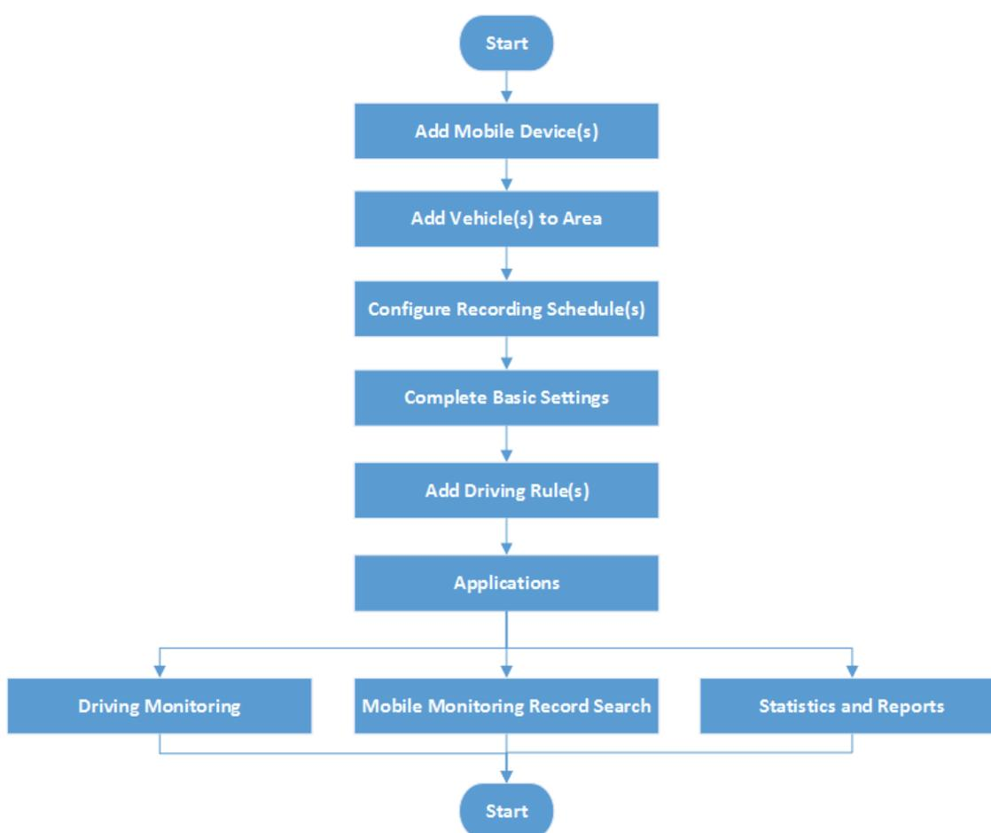
Figure 15-1 Flow Chart of Mobile Monitoring Configuration
