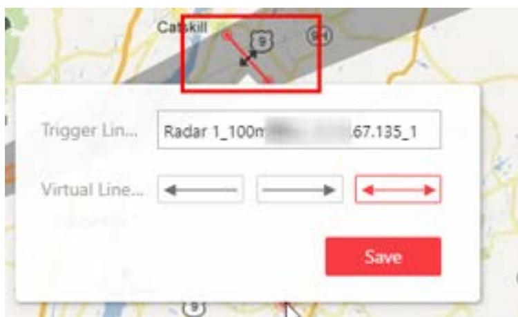
**Figure 28-3 Trigger Line in the Detection Area**
