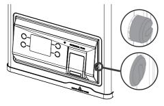
Ensure the red lock button on the right hand side of the control panel is in a depressed position. If not, push the button and simultaneously rotate it 90°. The button should remain depressed.
