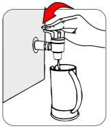
Push to lock for continuous flow. If lever does not lock, rotate it 180° before dispensing.
