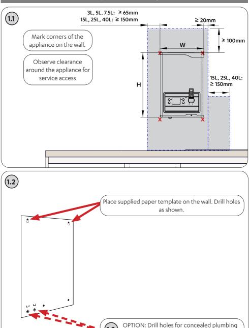
(water inlet, vent outlet) and electrical.
