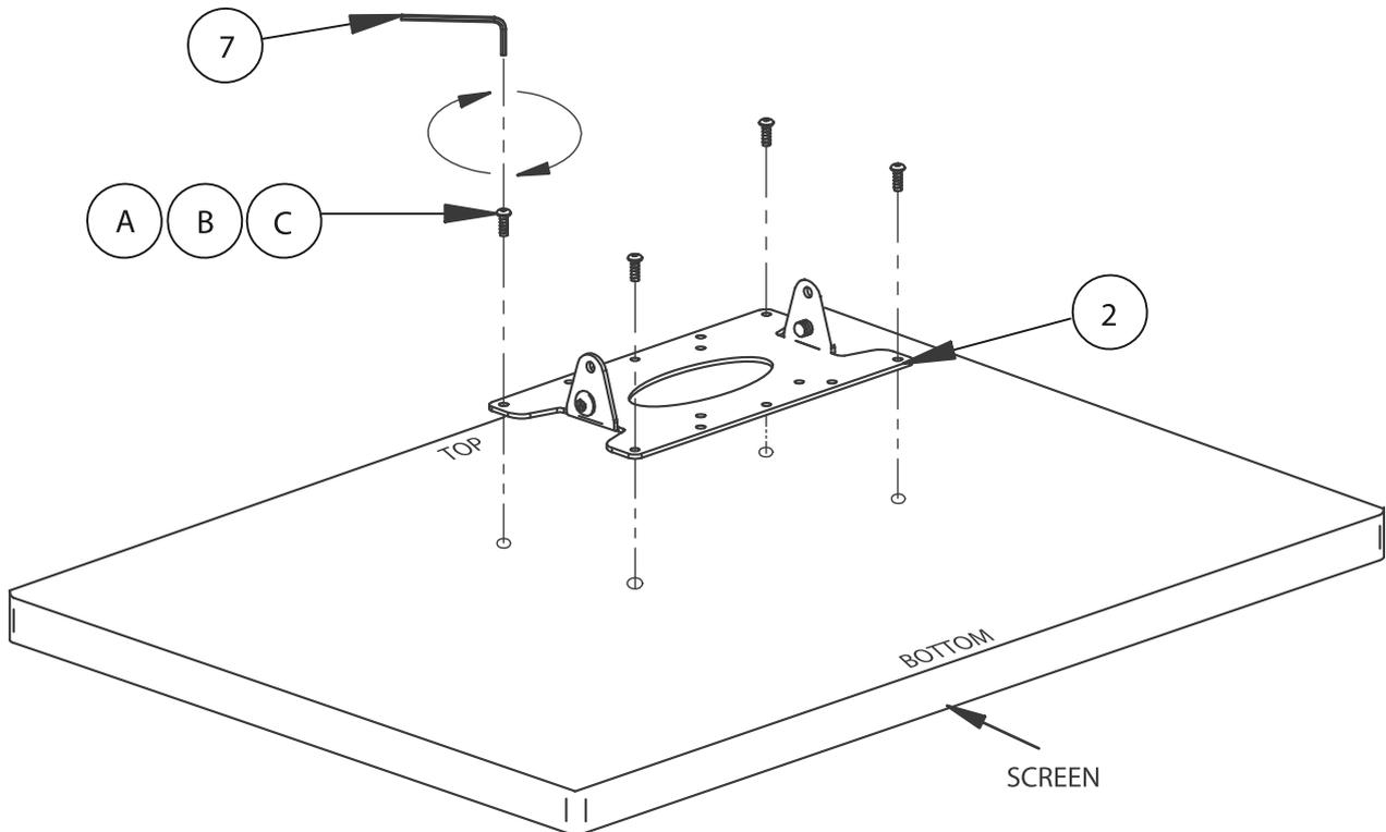
**Note:** Use M8 to M4 adaptors for screens with M8 fixings
