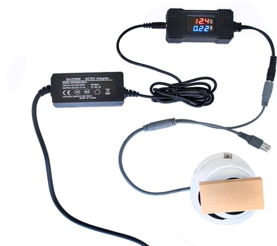
Fig 2 Shows camera current and voltage where IR is activated on camera
