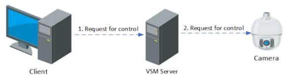
Figure 3-5 Flow of PTZ Control
