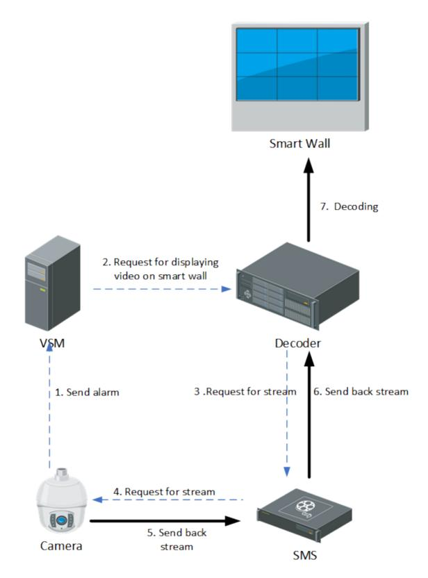
Figure 3-17 Flow of Displaying Alarm Video on Smart Wall via Streaming Server
