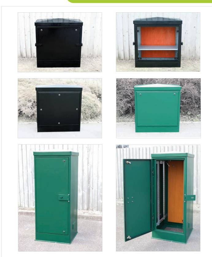
Our standard range of cabinets are of robust and secure design. They are not intended to compete with light duty pressed steel cabinets. Material used in the body is steel plate, which is between 4-6mm thick depending on cabinet size. All cabinets are fully fabricated and then hot dip galvanised after fabrication. The finish is powder coated, and the minimum expected life span is 25 years.
