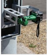
DSB - Drill Support Bracket, with Drill winder located in bracket
