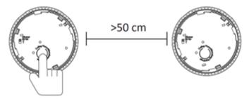
Turn on the power for the second detector as shown below.
