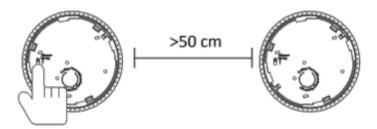
Now you will need to short press the coding button on the bottom of the first detector, The red LED will then flash slowly on the unit when it does release the button.
