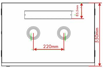
Colour: Black RAL9005 **Loading capacity:** 40kg Useable Depth: 315mm
