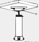
B: Fasten the snap joint fixing screw
