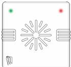
To set/unset the system using the external tag reader, present a pre-programmed tag to the centre of the device.
