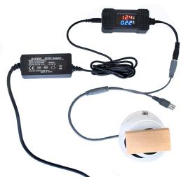
Fig 1 Shows camera current and voltage in normal mode
