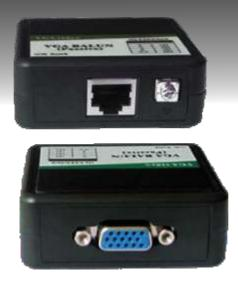
Plug your VGA cable from the VGA output into the Transmit Baluns HD15 connector. Secure the cables using the lock down screws. Make a similar connection between the Receive Baluns HD15 connector and your display. Insert the CAT5 cable into both ends of the Baluns. You may use standard EIA 568A/B termination.
