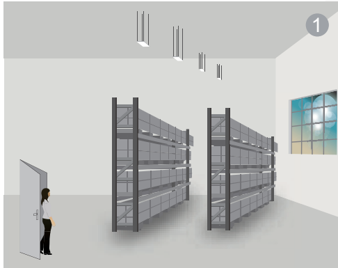
The light keeps off during daytime even when movement is detected. (Ambient lux level is above preset daylight threshold).
