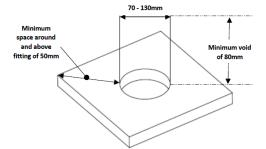
• This fitting will suit 70mm - 130mm cut-outs when using the adaptor ring (see Fig. 2)
