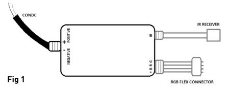
$\bullet$  Ensure the RGB Flex does not exceed the maximum wattage of the LEDFR4 controller
